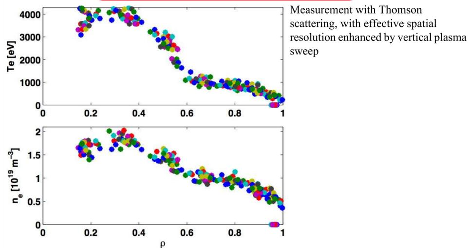
Measurement with Thomson scattering, with effective spatial resolution enhanced by vertical plasma sweep
