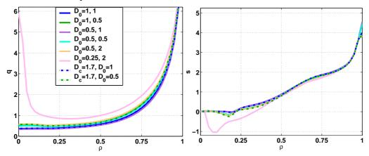
**FIGURE 6.** Astra results for TCV shot 31188 @t=1.4s: q-profile (left) and magnetic shear (right).
