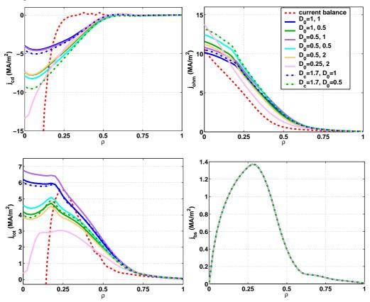
**FIGURE 5.** Astra results for TCV shot 31188 @t=1.4s: CQL3D  $j_{cd}$  (top left), ASTRA  $j_{ohm}$  (top right), ASTRA  $j_{tot}$  (bottom left), ASTRA  $j_{bs}$  (bottom right). The current balance values are experimental estimates of the different current density profiles, except for the  $j_{cd}$  which is calculated from linear theory.
