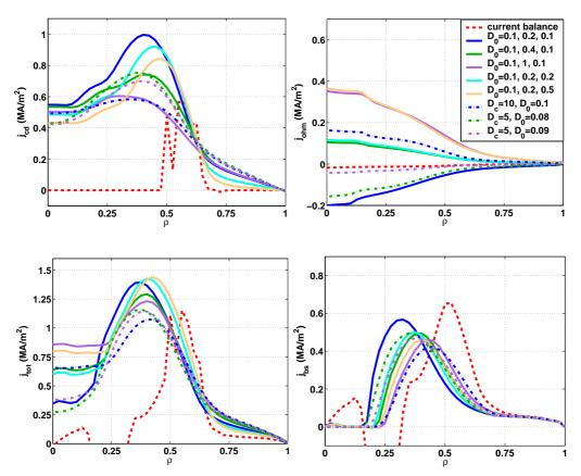
**FIGURE 2.** Astra results for TCV shot 28873 @t=1.15s: CQL3D  $j_{cd}$  (top left), ASTRA  $j_{ohm}$  (top right), ASTRA  $j_{tot}$  (bottom left), ASTRA  $j_{bs}$  (bottom right). The current balance values are experimental estimates of the different current profiles, except for the  $j_{cd}$  which is calculated from linear theory.
