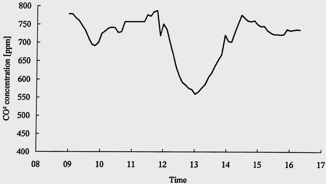
Figure H1: CO 2 concentration versus time. Morning coffee break and lunch time result in clear decreases of concentration.
