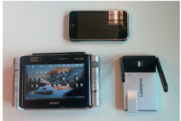
Figure 3. UMPC Sony VAIO UX90 and Linksys WUSB200. The scale is given by the iphone
