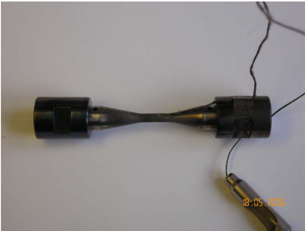
Figure 3. Specimen N29F26 shown after test. The main crack is on the left side of the gauge length.
