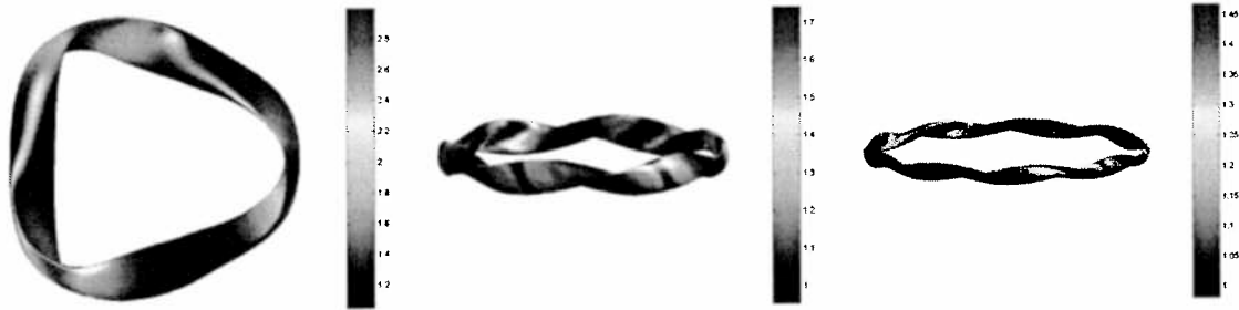
Fig.1. Boundary magnetic surfaces of the optimized N = 3 , N = 6 and N = 9 configurations. The color corresponds to the magnetic field strength on the boundary magnetic surfaces.
