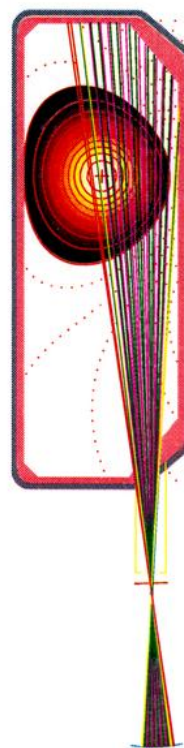
Fig. 1 Geometry of hard X-ray camera. The chords are partially overlapped.
