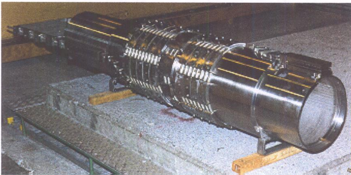
Figure 3 The winding, prepared for the heat treatment
