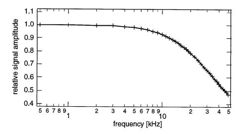
FIG. 4. Frequency response of the Hall probe system measured at a magnetic field of  $10\mathrm{mT}$ .
