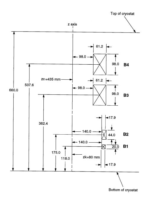
FIG. 5. Superconducting coil configuration used for calibration of the Hall probe as well as for different field properties. All dimensions are in mm. The coil current densities of the 4 coils  $B_1$  to  $B_4$  are  $I_1$  =115.248 A/mm<sup>2</sup>,  $I_2$  = -153.803 A/mm<sup>2</sup>,  $I_3$  =120.588 A/mm<sup>2</sup>,  $I_4$  =118.530 A/mm<sup>2</sup>, respectively.
