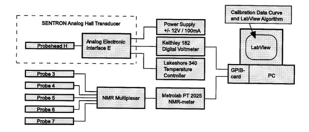
FIG. 1. Magnetic measurement set-up including Hall transducer, power supply, voltmeter, temperature controller and PC.
