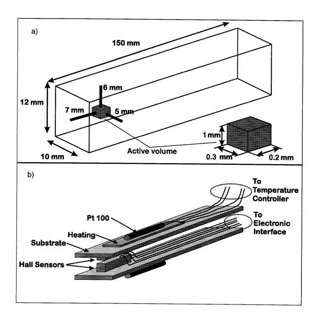
FIG. 2. Figure a). Overall layout of the probe head with details of the position and volume of the avtive part. Figure b) Details of the probe head: two Hall sensors are mounted on ceramic substrates as support plates, the heating foils are fixed on the outside and the standard 100W RTD platinum temperature sensors are fixed on top of these.
