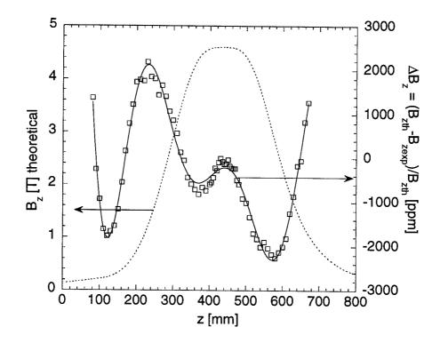
FIG. 8. Dotted line is the calculated on axis field  $B_z(z)$  and the squares are the relative difference between theory and experiment.
