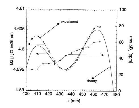
FIG. 9.  $B_z(z)$  component measured of axis at a radius of r = 25mm (squares). The continuous line is the theoretical value. The diamonds indicate the rms value taken on 6 different azimuthal positions (every  $60^{\circ}$ ) at each z-position.
