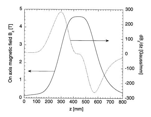
FIG. 6. Calculated on axis magnetic field  $B_z(z)$  and gradient  $\partial B_z/\partial z$  for the coil configuration shown in figure 5.
