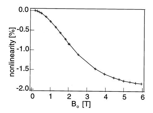
FIG. 3. Measured Hall probe sensitivity versus magnetic field.
