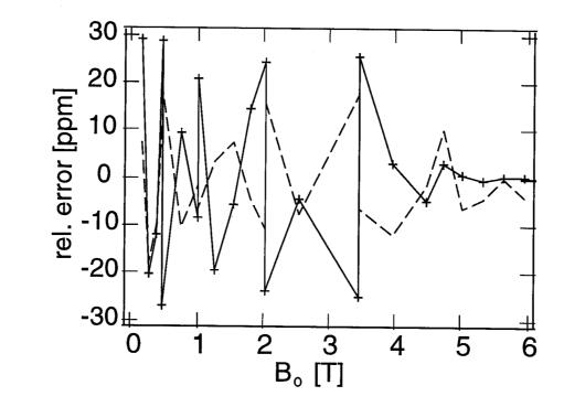
FIG. 7. Relative deviation between the magnetic field value measured with the NMR meter and Hall data corrected by the polynomial fit. This measurement has been performed with both probes placed in the homogeneous part of the magnetic field.
