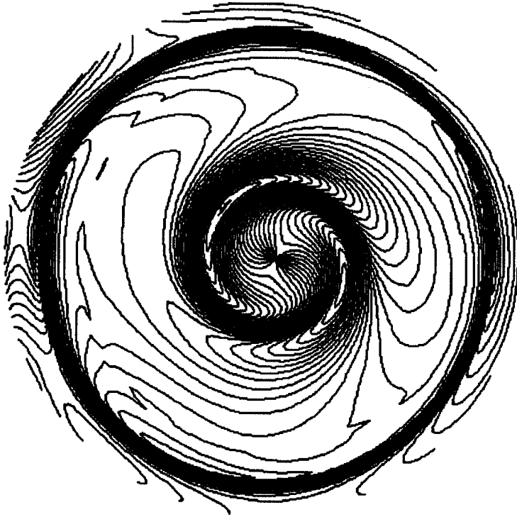
Figure 1: Level line plots for Re(E_n) using the LION code (zero Larmor radius model). The parameters correspond to the TCA tokamak with f = 2.45\text{MHz} , n = -2 , q_0 = 1.05 , q_a = 2.66 , B_0 = 1.5\text{T} , n_D = 5.2 \times 10^{19}\text{m}^{-3}(1 - 0.6s^2)
