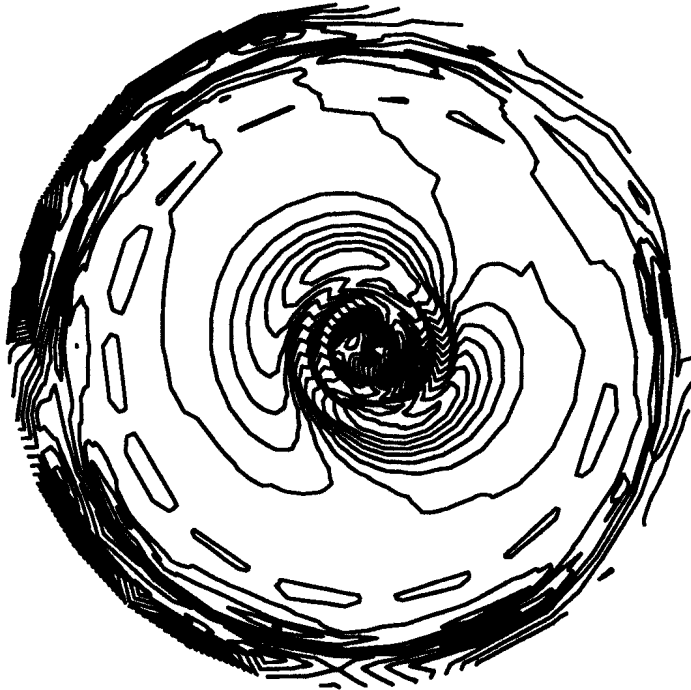
Figure 2: Level line plots for Re(E_n) using the PENN code (FLR model). The parameters are the same as in Fig.1, with T_e(s) = 400eV(1 - 0.98s^2)^2 , T_i(s) = 100eV(1 - 0.98s^2)^2 .
