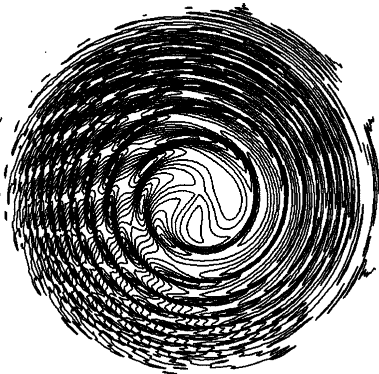
Figure 5: Level line plots for Re(E_n) using LION. The parameters correspond to the Phaedrus-T tokamak with f = 7\text{MHz} , n = -7 , q_0 = 1.5 , q_a = 3.8 , B_0 = 0.7\text{T} , n_{H0} = 0.3 \times 10^{19}\text{m}^{-3}
