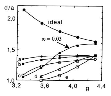
Figure 3. Marginal wall distance versus Troyon factor g for the plasma mode (marked "ideal") and the resistive wall mode using different assumptions. Curves (a - e) apply for  $\omega_{rot}/\omega_A = 0.06$ . (a - b) give results for the pressure damping model (1) with (a)  $v/\omega_A = 0.025$  and (b)  $v/\omega_A = 0.0025$ . (c-e) give results for the parallel viscosity model (2) with (c)  $\kappa = 0.1$ , (d)  $\kappa = 0.885$ , and (e)  $\kappa = 1.77$ .
