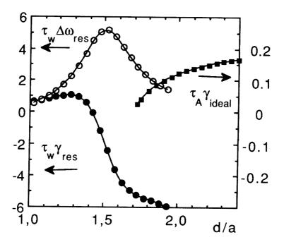
Figure 1. Growth rate  $\gamma_{res}$  and slip frequency  $\Delta\omega_{res} = \omega_{rot} - \omega_{res}$  of resistive wall mode and growth rate of plasma mode  $\gamma_{ideal}$  versus wall radius for n=1 mode with g about 30 % above free-boundary limit. This graph was calculated using the Hammett-Perkins approximation with  $\chi = 2/\pi$ .
