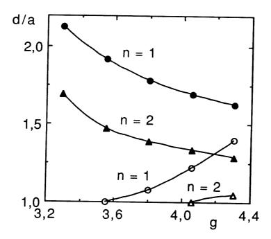
Figure 2 Marginal wall position versus Troyon factor g for the plasma (filled symbols) and resistive wall modes (open symbols) with toroidal mode numbers n=1 and n=2. The plasma mode is stable for  $d < d_{crit}$  and the resistive wall mode for  $d > d_{crit}$ . The region stable to both the n=1 and n=2 modes is bounded by the n=1 resistive wall mode and the n=2 plasma mode.
