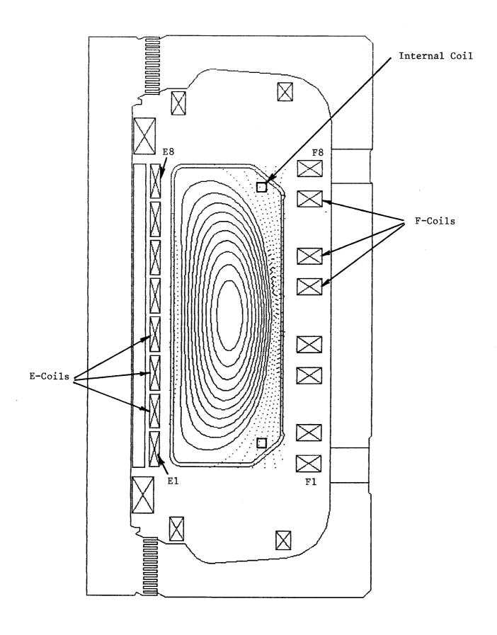
Fig.1. Cross Section of TCV Tokamak
