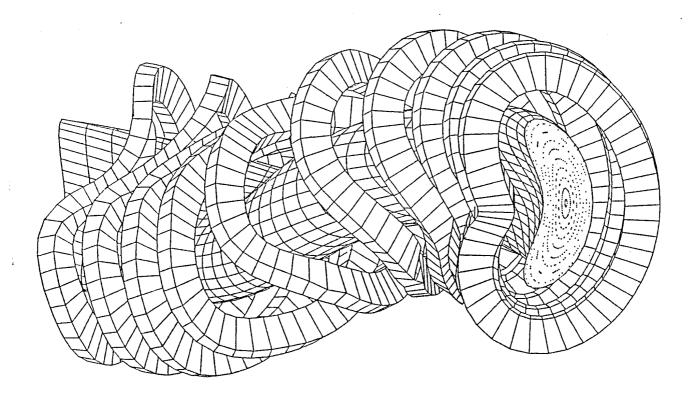
Fig. 1. The magnetic field coil structure and the plasma shape in one field period of a 4 field period Helias stellarator configuration. The cross sectional cut shows the shape of the internal flux surfaces in the plasma obtained by puncture plots left by the intersection of magnetic field lines traced over many toroidal transits across the plane defined by the cut.
