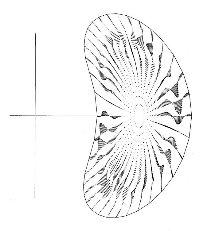
Fig. 3. The flow pattern corresponding to the most unstable eigenmode structure at the toroidal plane with Boozer coordinate toroidal angle  $\phi = 0$  in a 4 field period Helias stellarator configuration. The structure is dominated by an m = 4, n = 3 mode concentrated about the  $\iota = 0.75$  surface. The configuration has a plasma  $\beta = 2\%$  and zero net toroidal plasma current within each flux surface.
