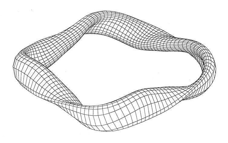
Fig. 2. The full 3D structure of a flux surface corresponding to a 4 field period Helias stellarator configuration.
