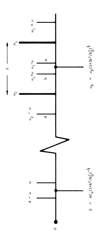
Schematic representation of the high and low frequency spectra associated with two high frequency pumps at the frequencies  $\omega_1$  and  $\omega_2$ with a separation  $\Delta$
