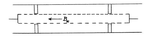
be limited with the aid of quartz diaphragms and an axial magnetic field  $B_z \sim 3-5$  kG (large enough so that the ion Larmor radius is small compared with the column size). The z-rf circuit could be modified (Lietti 1973) to give  $I_z \sim 20$  kA through the plasma load of inductance L  $\sim 250$  nH.
