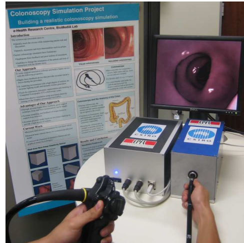
Figure 1: The colonoscopy haptic device is highly portable and rugged. Shown with an Olympus CF-160 colonoscope inserted, and the MILX™ GastroSim framework rendering a colon model extracted from CT colonography [3]
