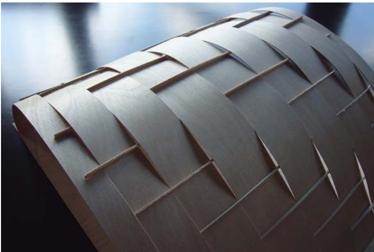
Fig. 9 Woven timber structure
