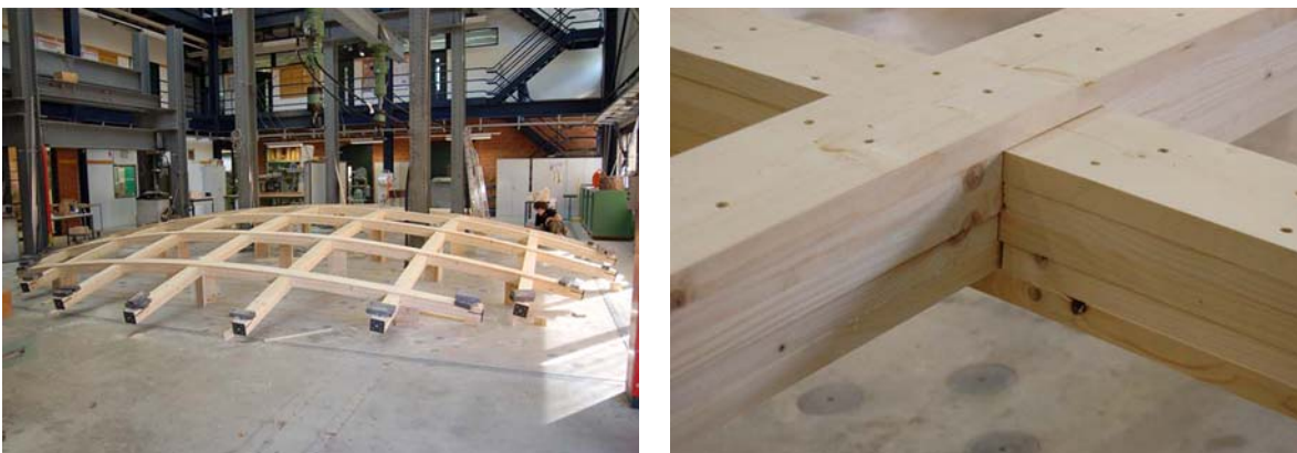
Fig. 7 Experimental Rib Shell Structure
