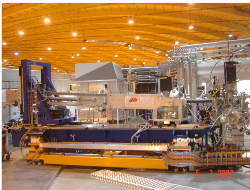
Figure 2.1: Photo of SAXES spectrometer installed at SLS ADRESS beamline.
