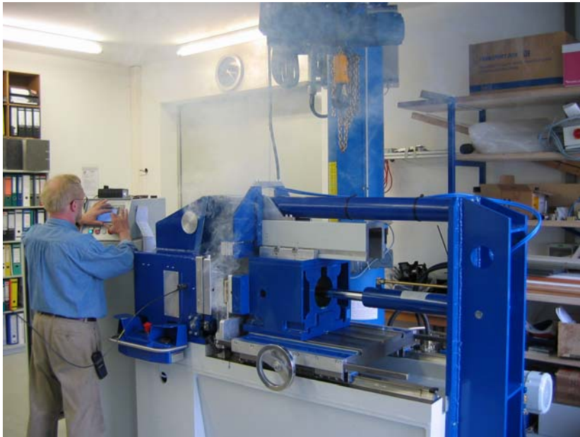
Figure 5 : Friction welding machine conceived especially for wood during a welding test. Welding is accompanied by smoke generation.
