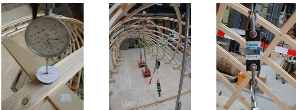
Fig 5 Load tests; uniaxial displacement transducer (left); loading with two single loads (center); load measuring (right)
