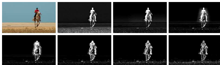
Fig. 3. From left to right, original image followed by filtered images. Filtering is done using R_1 of size one pixel and varying width of R_2 . When R_2 has the maximum width, certain non salient parts are also highlighted (the ground for instance). It is the saliency maps at the intermediate scales that consistently highlight salient regions. The last three images on the right mainly show edges.
