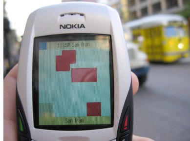
Figure 4. Display of Jabberwocky, providing a quick way to visualize the current and past strangers encountered. Newly encountered strangers appear at the top of the screen as red squares. As time elapses, the strangers slowly move down towards the bottom of the screen. Once they reach the bottom they slowly fade out.
