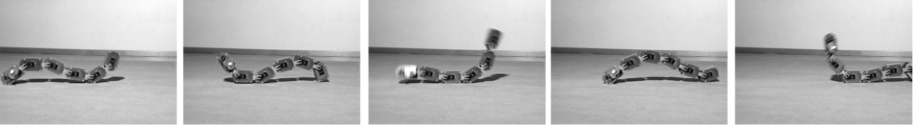
Figure 13: Snapshots of a learned gait in the snake robot. The robot is propelled by a traveling wave going from tail (left end with LED marker) to head.
