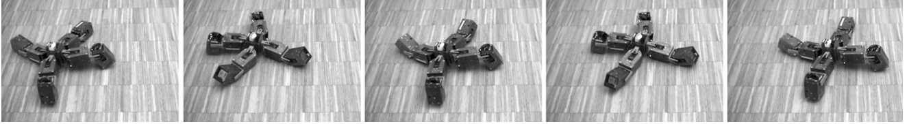
Figure 20: Snapshots of the learned gait in the quadruped robot. The center of the robot describes a zig-zag trajectory in the horizontal layer (with two steps per cycle).
