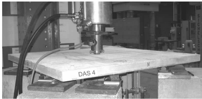
Figure 6.9: Thin UHPFRC slab without ordinary reinforcement subjected to bending test under point load
