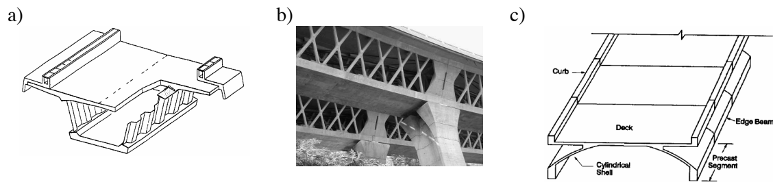
Figure 7.10: Possible solutions for a light UHPFRC superstructure for higher spans: a) corrugated webs (as in the Altwipfergrund bridge, mixed design); b) voided webs – truss structures, Glacières and Sylans viaducts, 1988-89, France; c) shell-deck bridge [Fanous et al. 1996]
