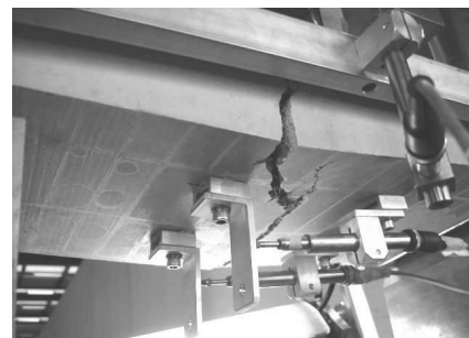
Figure T.5: Measuring devices: a) LVDT_01, measuring vertical displacement; b) LVDT_02 and LVDT_03 measuring horizontal elongations
