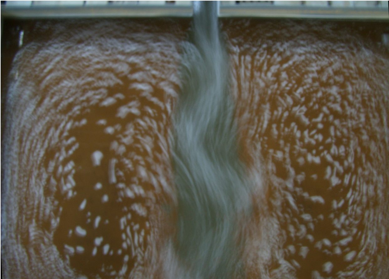
Figure 2.4: Plan view of the particle streaks and vortex street-like instability of a shallow turbulent wake flow in a rectangular reservoir at LCH. Visualization by introducing particles on the surface.
