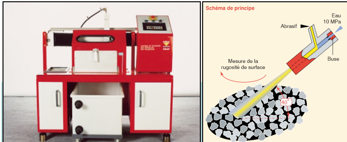
Figure 3: Machine GRAP – principe (source: www.lcpc.fr)
