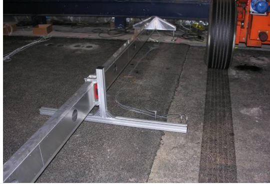
Figure 2: Specific deflection beam used in the ALT facility
