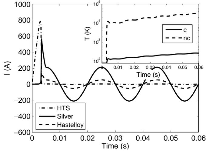
**Figure 3.** Distribution of the current ( $I_{peak}=810$  A) in the tape materials for a shunted tape (substrate and stabilizer). The inset is the temperature of the tape for a shunted (c) and non-shunted (nc) device. For a non-shunted configuration, all the current goes in the HTS which has a high resistivity in the normal state. This has a direct effect on the temperature increase.
