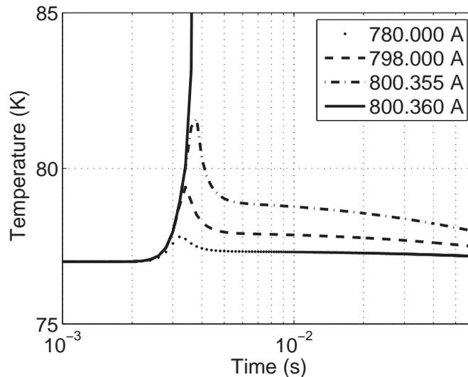
**Figure 2.** Effect of the current on the thermal stability. A threshold current around 800 A is observed for this model.
