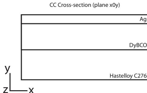
**Figure 1.** Cross section of the simulated CC (not drawn to scale). The tape is 10 mm wide and is composed of three layers: 1) Hastelloy substrate (1.8 mm), 2) DyBCO film (60  $\mu\text{m}$ ) and 3) an Ag stabilizer (60  $\mu\text{m}$ ). We intentionally omitted the MgO buffer layer to reduce the computation time.
