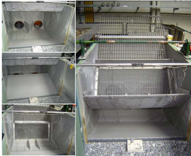
Figure 3.3: LEFT: Outlet pipes (top), tilting gate (center), sediment sampling device (bottom), RIGHT: general view of the outlet box
