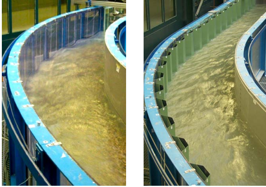
Figure 4.19: Water surface waves with the smooth wall (left) (picture taken from Hersberger [1]) and the undulated wall (right) 1
