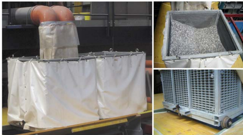
Figure 3.4: LEFT: Outlet pipes and filtering baskets with the skirts against splashing, RIGHT: filtering basket with the sediments (top), double grid, closing mechanism, wheel and rails (bottom)
