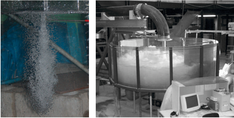
Figure 3.9.: Left: free jet diffusion (Chanson et al., 2004), D = 12.5 mm, V = 3.3 m/s, freshwater (courtesy of Dr Hubert CHANSON); Right: Plunging jet diffusion in a flat shallow pool, D = 72 mm, Y/D = 5.6 , V = 20 m/s.
