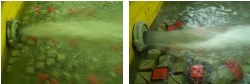
Figure 15: View of a high discharge with low and high tailwater level, Test Hb10 - 215 (above), Test LB10 - 215 (below) – Q = 21.5 l/s
