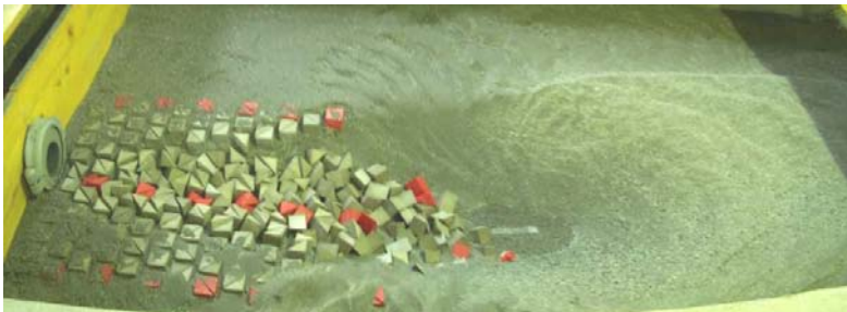
16 – Test M"b10 - 185, Q = 18.5 l/s, h_{TW} = 7.20 cm (Failure)
