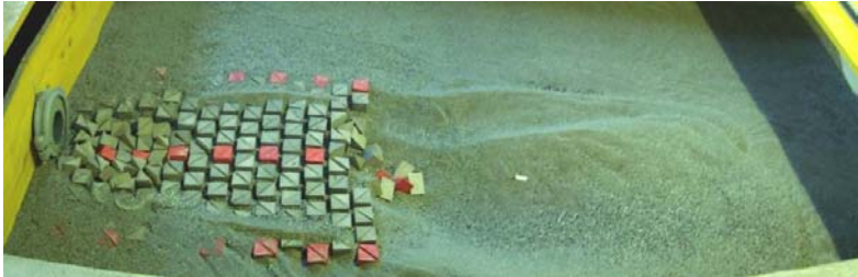
13 – Test M'b10 - 125, Q = 12.5 l/s, h_{TW} = 5.00 cm (Acceptable movement of prisms)
