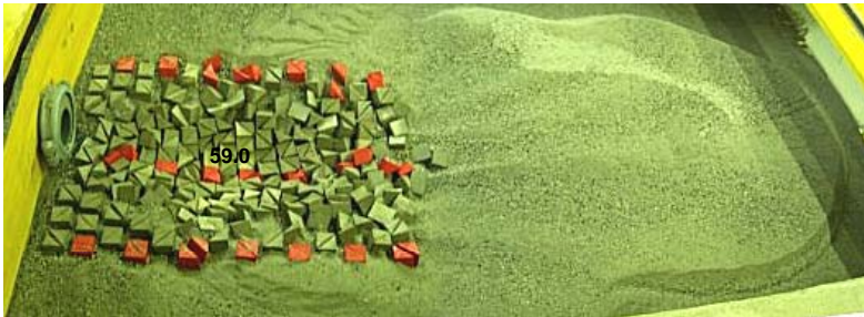
10 – Test Lb10 - 155, Q = 15.5 l/s, h_{TW} = 1.90 cm (Acceptable movement of prisms)
