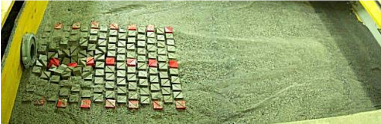
7 – Test Lb10 - 50, Q = 5.0 l/s, h_{TW} = 0.90 cm (Acceptable movement of prisms)
