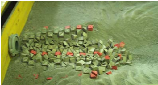
14 – Test M'b10 - 185, Q = 18.5 l/s, h_{TW} = 5.70 cm (Failure)
