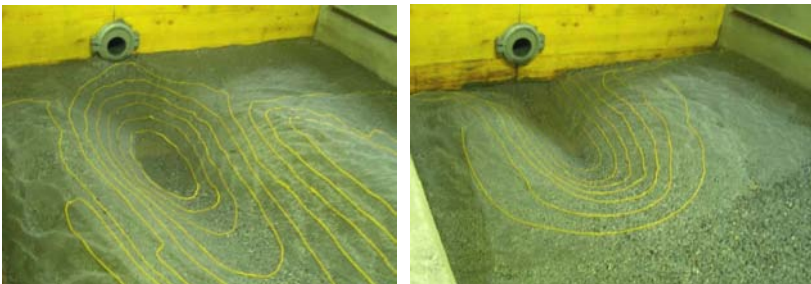
Figure 17: Test HN10-125, high tailwater depth (left), Test LN10-125, low tailwater depth (right) – Q=12.5 l/s
