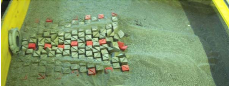
15 – Test M"b10 - 125, Q = 12.5 l/s, h_{TW} = 6.50 cm (Acceptable movement of prisms)
