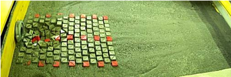
8 – Test Lb10 - 80, Q = 8.0 l/s, h_{TW} = 1.40 cm (Acceptable movement of prisms)
