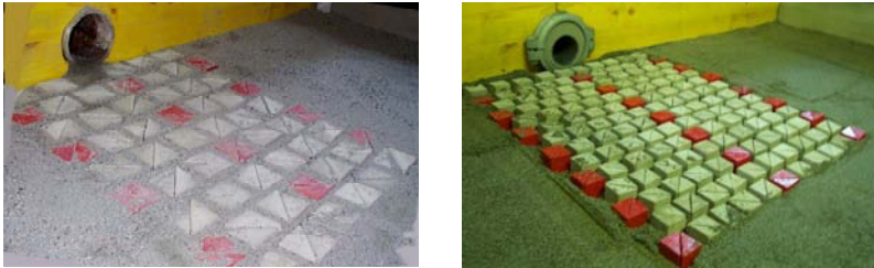
Figure 12: View of the downstream protected area, prisms 8 cm (left); prisms 5 cm (right)
