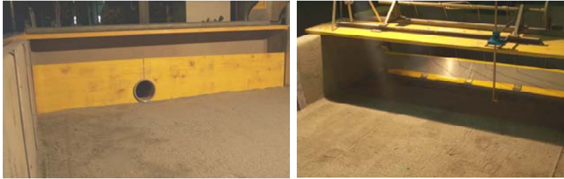
Figure 11: Alluvial bed; view towards upstream (left), view towards downstream, tailwater flip gate and point gage (right)
