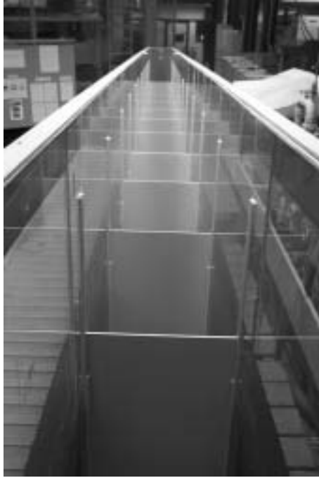
Figure 3.13: Photograph of the flume divided for the calibration
