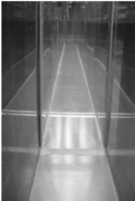
Figure 3.21: Photograph of the water jet injection apparatus.
