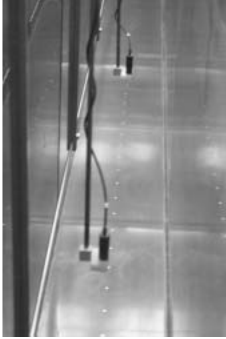
Figure 3.8: Photograph of the UVP transducer as well as the bottom and reference electrodes.
