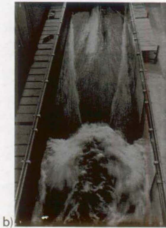
Fig. 2.2 : Flow downstream from abrupt expansion. a) supercritical flow throughout; b) jump in the proximity of overflow weir. i) plan view; ii) axial section; iii) section near side wall.
