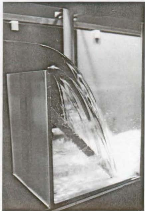
Fig. 4.13 : Discharge measuring devices used in LCH1. a) 90 deg. V-notch sharp-crested weir; b) rectangular sharp-crested weir.
