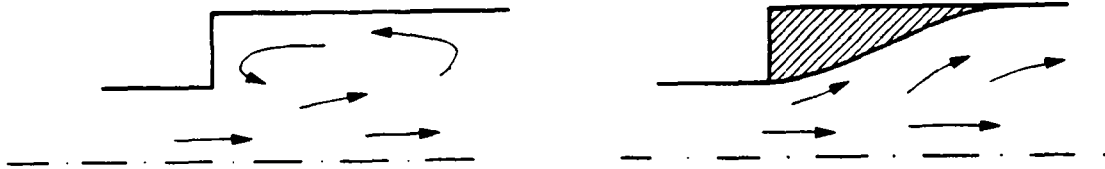
Fig. 3.7 : Side element by which the formation of a lateral eddy is suppressed (Herbrand 1971).
