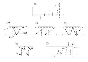
Fig. 5—Development of actual cracking pattern: (a) initial flexural cracks; (b) cantilever action; (c) aggregate-interlock action; (d) dowel action; (e) tensile stresses due to (b-d); and (f) final crack pattern.
