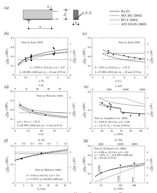
*Fig.* 13—*Comparison of Eq.* (5), *SIA* 262,<sup>14</sup> *EC-2*,<sup>39</sup> *and ACI* 318-05<sup>24</sup> (*corrected by ACI* 440.1*R*-01<sup>40</sup> *in plot* (g)) *for various cases:* (a) geometrical and mechanical parameters; (b) and (c) tests by Kani;<sup>18</sup> (d) and (f) tests by Walraven;<sup>28</sup> (e) tests by Angelakos et al.;<sup>9</sup> and (g) tests by El-Sayed et al.<sup>41</sup> with steel, carbon fiber; and glass fiber reinforcement.
