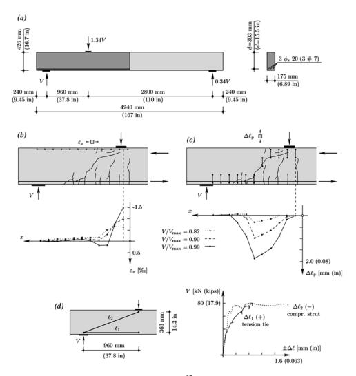
Fig. 8—Test BP0 by Muttoni and Thürlimann<sup>17</sup> ( $f_c = 30.5$  MPa [4.42 ksi];  $d_g = 16$  mm [5/8 in.]): (a) test setup; (b) crack pattern and horizontal strains along top fiber (points of measurement indicated); (c) crack pattern and vertical elongation along diagonal crack (points of measurement indicated); and (d) measured elongations in directions of compression strut and of tension tie.
