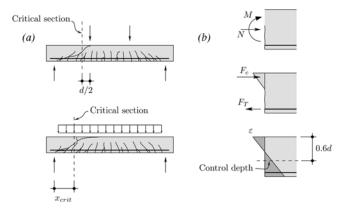
Fig. 9—Critical shear crack model: (a) critical section for point loading and distributed loading; and (b) determination of longitudinal strain in control depth using internal forces N and M.
