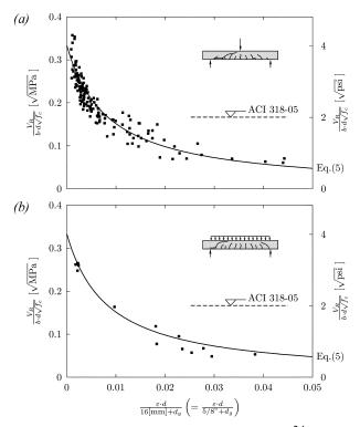
Fig. 10—Comparison of Eq. (5) and ACI 318- $05^{24}$  with test results for normal and high-strength concrete members: (a) concentrated loading; and (b) distributed loading.
