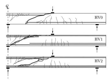
*Fig. 11—Cracking pattern in Beams HV0, HV1, and HV2*<sup>37</sup> with reinforcement cutoffs.
