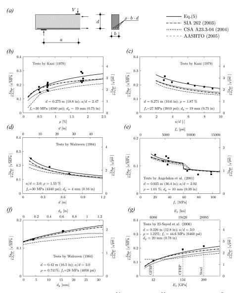
Fig. 14—Comparison of Eq. (5), SIA 262,<sup>14</sup> CSA A23.3-04,<sup>11</sup> and AASHTO LRFD<sup>8</sup> for various cases: (a) through (g) same geometry and tests as in Fig. 13.
