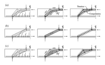
Fig. 6—Load-carrying mechanisms after development of critical shear crack: (a) elbow-shaped strut; (b) straight strut (enabled by aggregate interlock); and (c) combined response.
