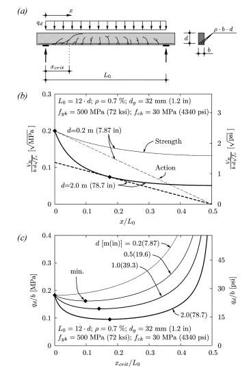
Fig. 12—Shear critical section for distributed loading: (a) geometry and mechanical parameters investigated; (b) location of critical sections (tangent between strength and action lines) for two effective depths; and (c) required load to develop shear failure at each section of beam and minimum (indicating shear critical section) for various effective depths.
