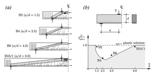
*Fig.* 4—Influence of a/d on shear strength: (a) Tests B2, B4, B6, and BP10/1 by Leonhardt and Walther,<sup>16</sup> cracking pattern and theoretical strut position; and (b) Kani's valley, comparing actual strength with failure load according to theory of plasticity.
