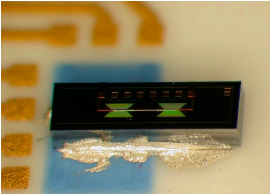
Figure 5.27: The sensor chip attached to the ceramic substrate with silver epoxy.
