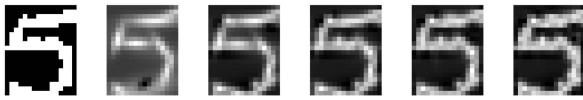
Fig. 2. Progressive OMP approximation of the digit “5” (leftmost) with 10, 20, 30, 40, and 50 Gaussian atoms (from left to right).
