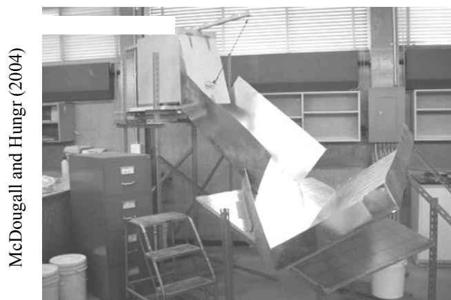
Figure 2-12 Experimental set-up of McDougall and Hungr (2004)
