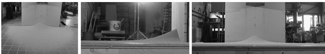
Figure 4-17 Test at 90^\circ slope; release of 40 l of gravel, from 1 m height, on a board covered with wood
