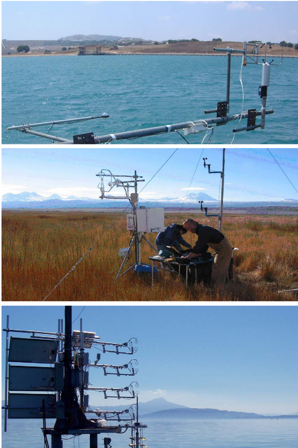
Fig. 1. Pictures from the three sites, illustrating the three different environments and experimental set-ups: Eshkol reservoir; Israel (upper); Tilopozo wetland, Chile (center); Lac Léman, Switzerland (lower). In the wetland, a 1-D sonic anemometer and a Krypton hygrometer were installed most of the time.
