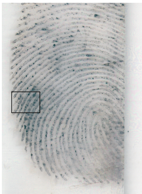
Fig. S1. An optical laser-scanner image of a MMD-enhanced latent fingerprint on the glass substrate. The SECM image area corresponds approximately to the rectangle region marked (inside black line), that is, the area in Fig. 2a.
