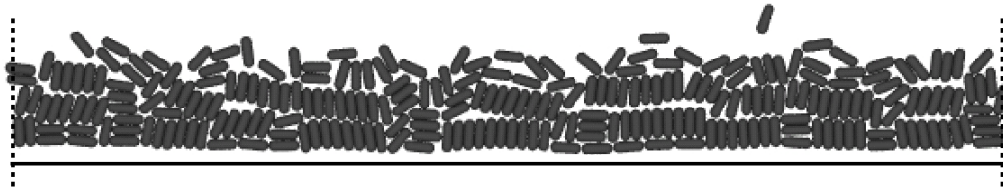
Figure 3.5: Simulations 4 - Rearrangement after 1200s of vibrations. Initially the particles were ordered horizontally. Lateral walls are periodic.
