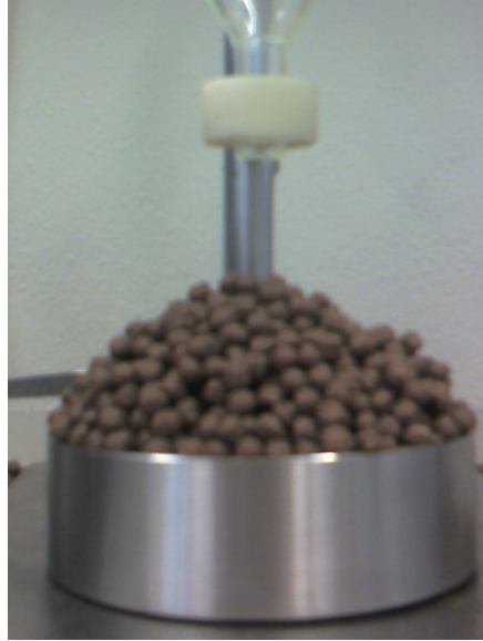
Figure 2.11: Image from an angle of repose test.
