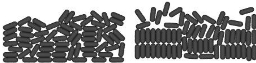
Figure 3.2: Simulation 1 - Starting configuration (left); positions of the particles during vibrations after 1200 s (right); the walls of the pseudo-two-dimensional box are omitted.
