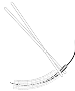
Fig. 3. Sliding an arc along a circular path is one of the dexterity primitives we use to learn maneuvering a needle in microsurgery
