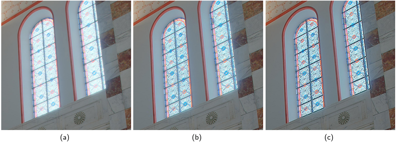
Figure 8. Illustration of sharpening and halo artifacts. (a) Image rendered with \sigma_H = 0.5 and \sigma_A = 1.5 . (b) Image rendered with \sigma_H = 1.5 and \sigma_A = 3 . The edges are sharper than in (a). (c) Image rendered with \sigma_H = 3 and \sigma_A = 4 . The sharpening effect is too strong and visually looks like halo artifacts along high contrast edges.
