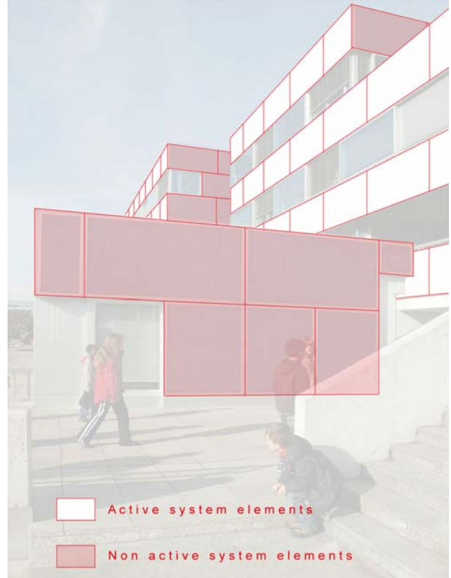
Figure 8 a: LESO glazing integration simulation over Pully school (CH); 8-b: Active and non active areas.
