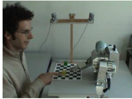
Figure 3: The robot imitates the human pointing to an object. In the background a stereovision system tracks the location of the objects and the demonstrator's hand
