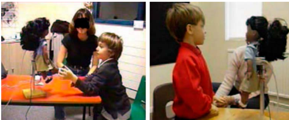
Fig. 2 Examples of trials from an early study with Robota [7]. In order for the robot to detect vertical arm movements performed by the children with autism a very restricted setup had to be used where the children needed to stay very close to the robot. The robot could only detect gross arm movements. It was observed that the children needed a lot of encouragement from the teacher. Teacher–child interactions were less playful and more instruction oriented.
