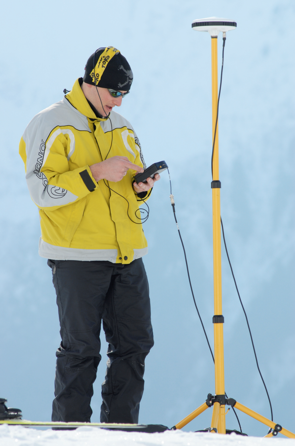
Engineer Stéphane Ducret, of TracEdge, calibrates the GPS reference receiver and mobile unit.
