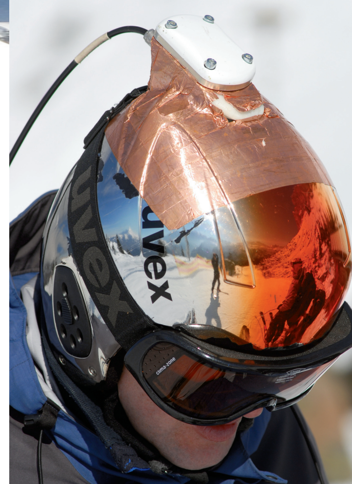
Jan Skaloud and GPS/INS-equipped helmet
