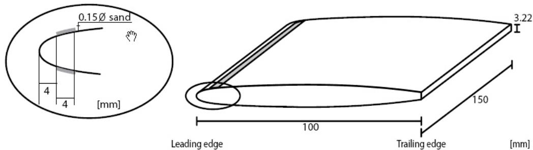
Figure 1. Blunt truncated Naca0009 hydrofoil and distributed roughness
