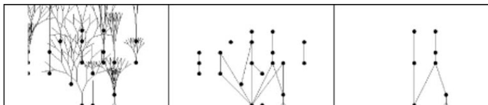
Fig. 6 Growth of axonal connections in the 2D brain space, pruning of axons that do not connect to other neurons, and pruning of all neurons that are not connected to input, output, or other parts of the network. From Nolp et al. [57]
