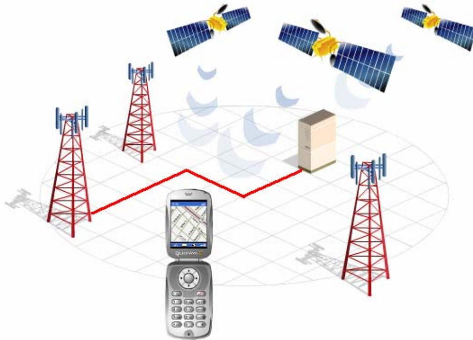
Fig. 2.11 Functional schema of AGPS technology (source Qualcomm).
