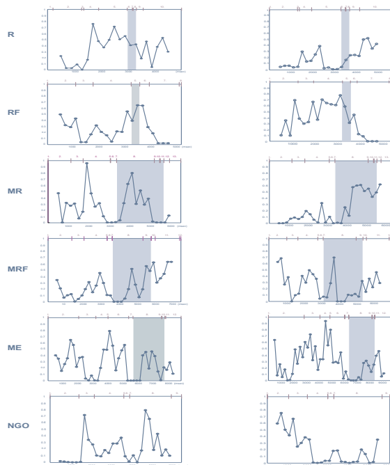
Figure 5: 'On-line' classification using the second method. Some examples. x axis - recording time, y axis - probability of finding motor intention in the data.
